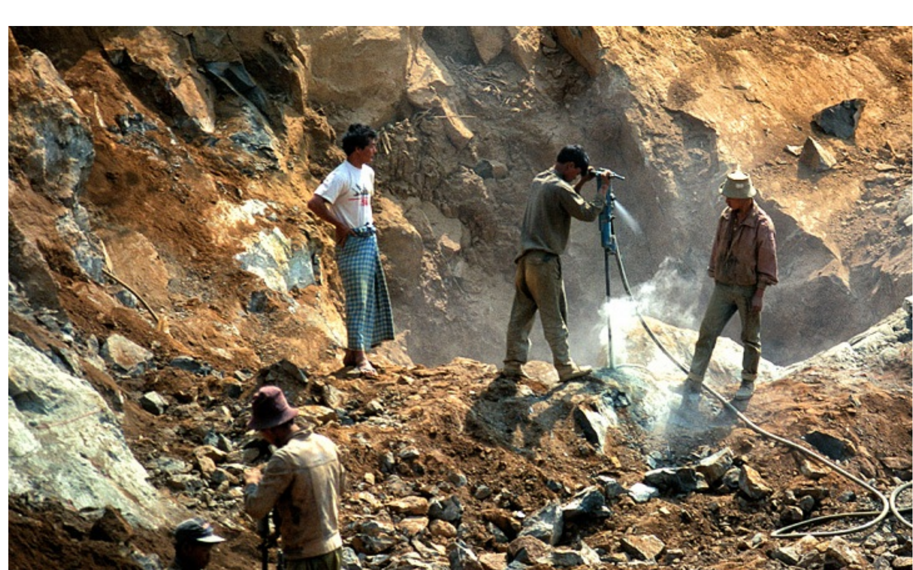
4.. Once a dike is exposed, miners use dynamite & jackhammers to break the jadeite apart.
