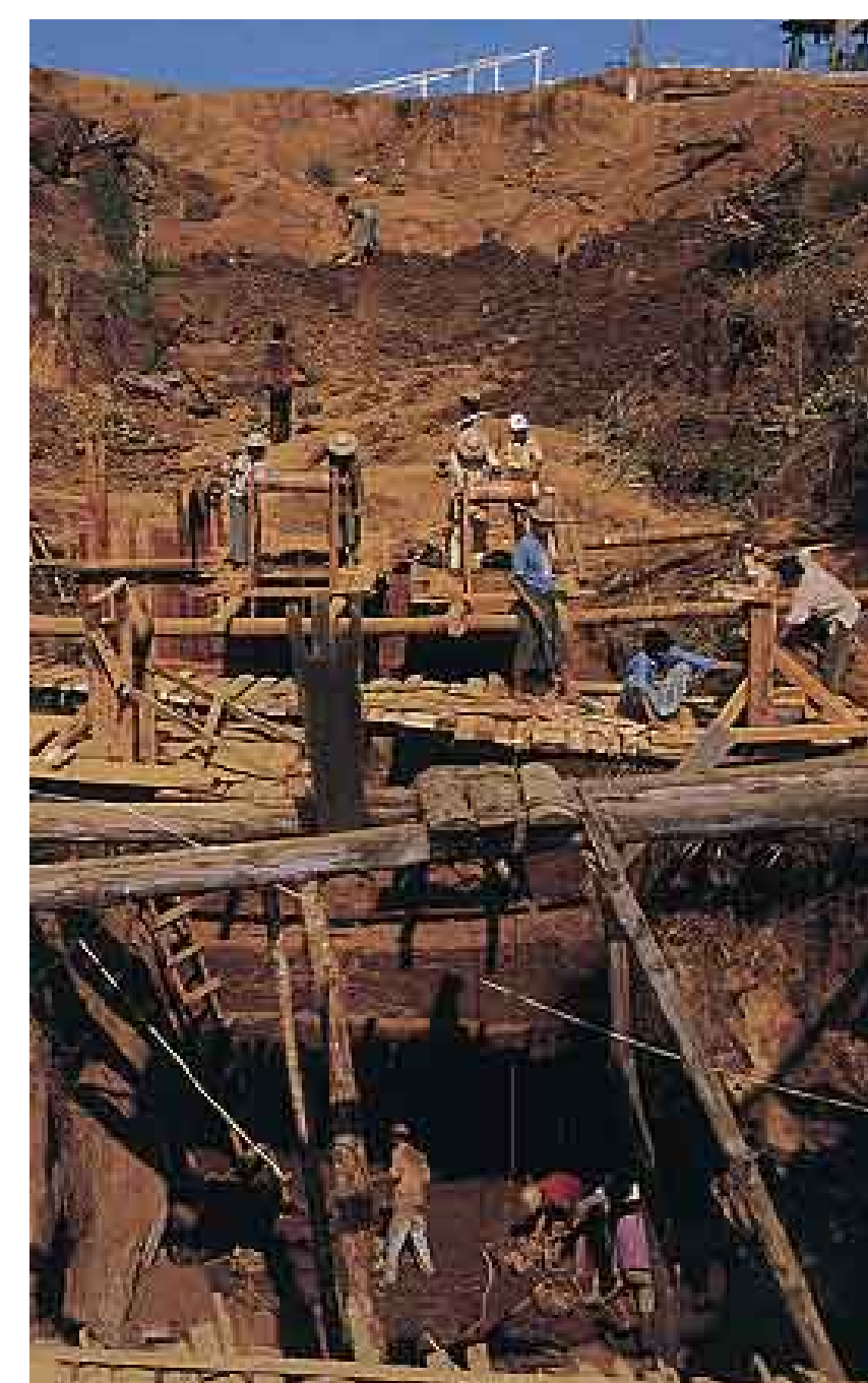
3.. Miners must dig deep shafts through the overden to reach the jadeite dikes. Dirt & gravel are removed by a rudimentary winch & bucket system.
